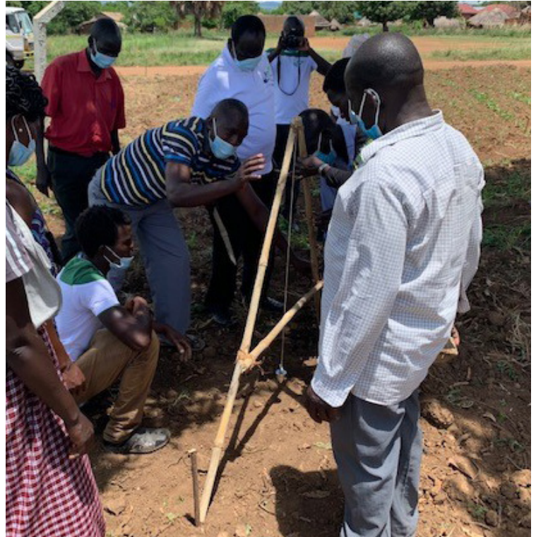
Alur farmers use an "A" frame level to find contour at the Agroecology Workshop in Nebbi, Uganda.
